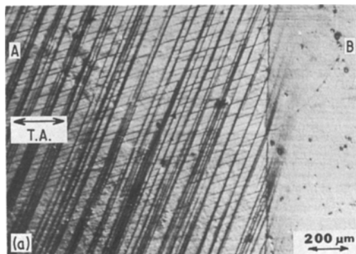
Figure 3 Coarse slip lines in the beta phase initiated by interaction of slip in alpha phase with a flat phase boundary. Cross-head speed is 0.005 \text{ cm min}^{-1} . Micrographs are of a region different from the one shown in Fig. 2 (a) At a stress level of 52.5 \text{ MN m}^{-2} (strain = 20.1%); (b) at a stress level of 60.4 \text{ MN m}^{-2} (strain = 26.9%).
